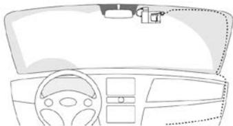
A safety critical event occurs (accident, hard brake, overspeed, panic button, alarm input). Device records HD video at full frame rate to its internal storage. At the same time, KP1S transmits a preview file and e-mail message to SmartMail server.
