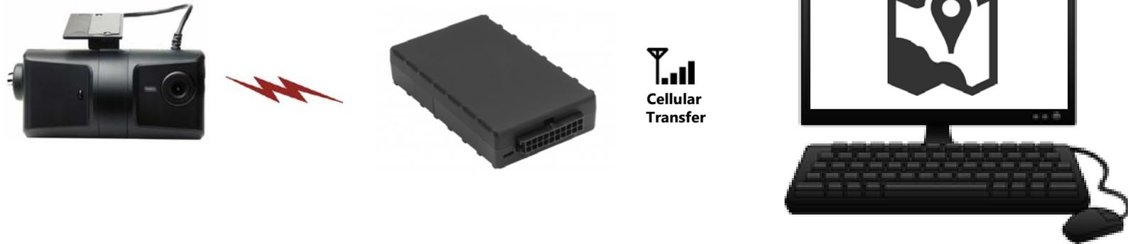
Upon event trigger, the SmartWitness device will send a notification via a telematics device installed in the vehicle. This will create an alert on the GPS tracking application which allows for auditing of camera events.
