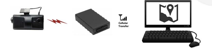
Upon event trigger, the SmartWitness device will send a notification via a telematics device installed in the vehicle. This will create an alert on the GPS tracking application which allows for auditing of camera events.
