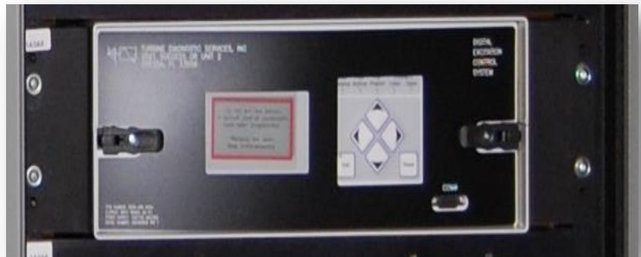
The **400 Series Digital Excitation Control System** is a microprocessor based controller that provides excitation control, flexible logic control and optional power plant system stabilization for synchronous machines in an integrated package. These are most often incorporated in upgrades for SCT/PPT, potential source SCR bridges, Amplidyne, ALTERREX, GENERREX and the larger brushless and rotating DC exciters.
