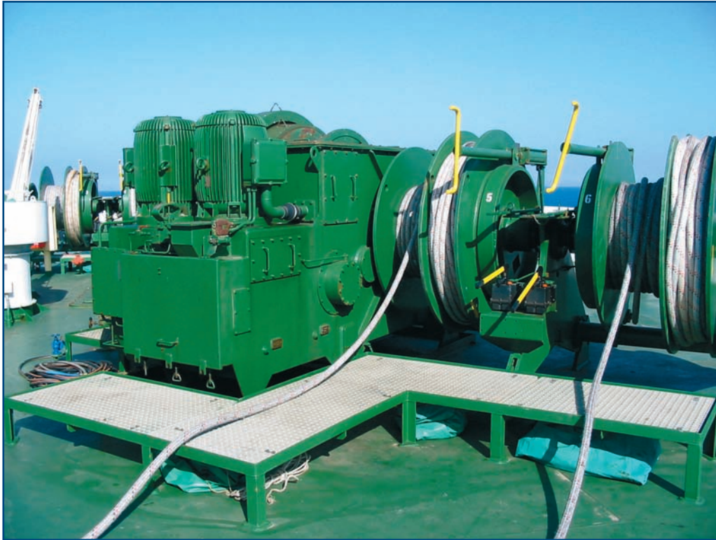
Figure 7.2: Jacketed High Modulus Fibre Moorings on Split Drum Winches
