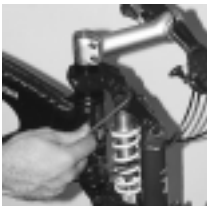
Top Shock Bolt Removal
