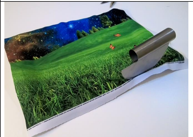
Insertion of the textile in the extrusion channel.
