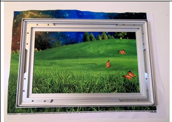
The frame is centered onto the chosen textile. Leave a minimum of 2" bleed all around the frame.
