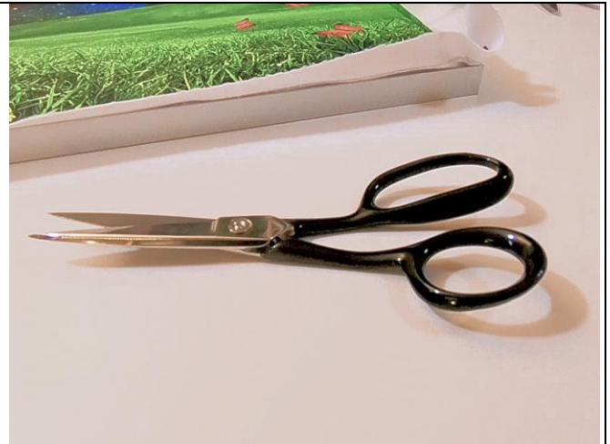
Cut extra textile (Bleed) with a very practical 8" shear
