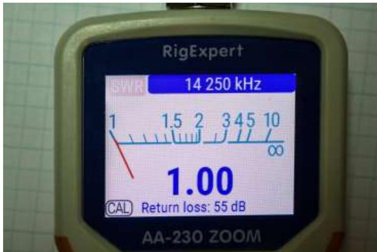
Typical SWR & Return loss for the SOL on a single frequency.
