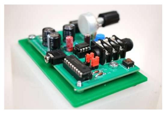
The trim potentiometer located between the key jack and volume control need not be touched and has been preset at production of this unit. Changing the position of this trimmer alters the drive from the oscillator to the amplifier and if needed can be adjusted to increase the output volume but is really only for access by our technicians. Altering this control will not damage the unit.
