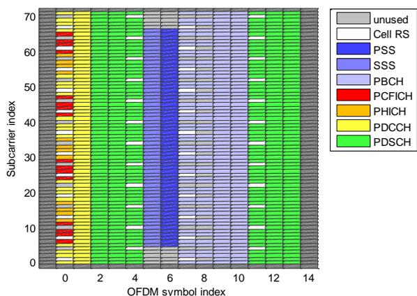
Fig. 1 Downlink transmit resource grid for a sub-frame
