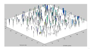
Fig. 2 Uplink transmit resource grid for a sub-frame
