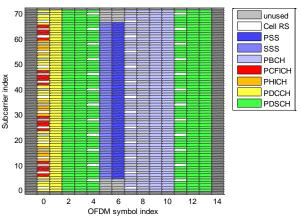
Fig. 1 Downlink transmit resource grid for a sub-frame
