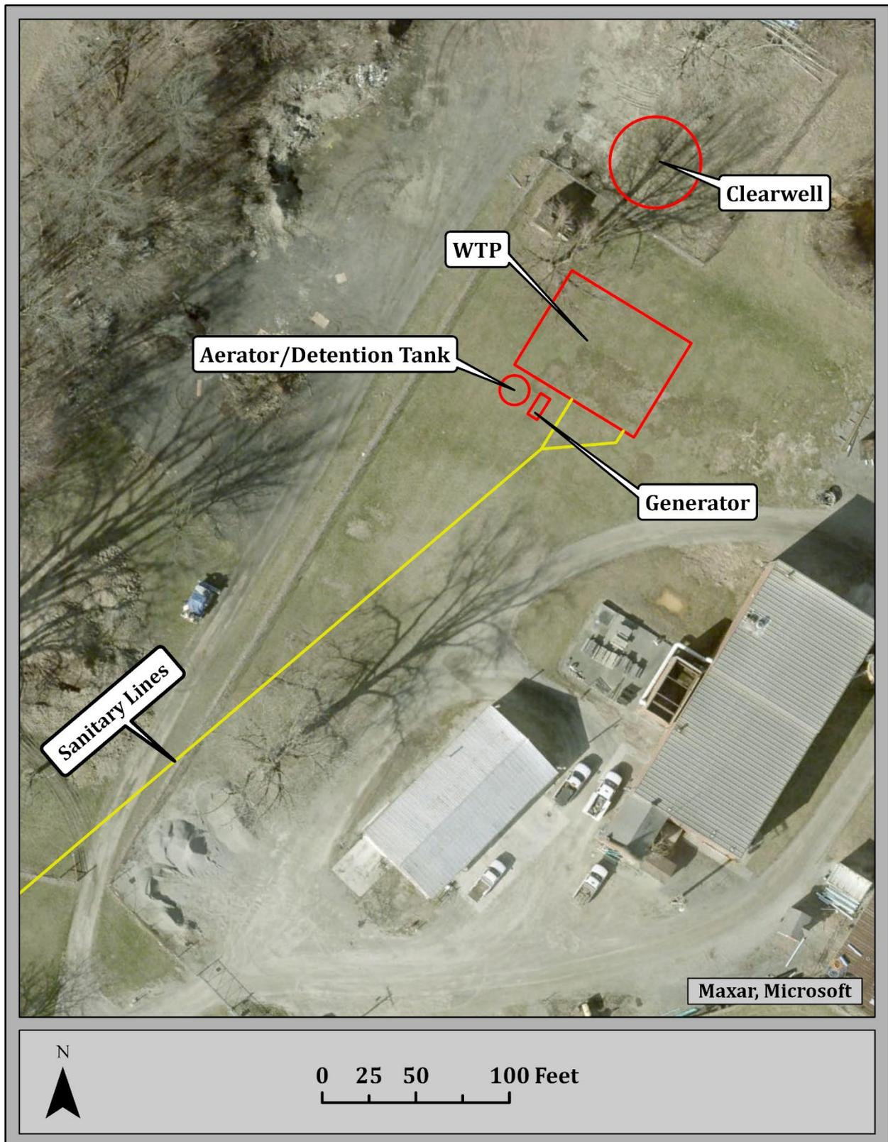
Figure 2. Location of proposed new WTP in relation to the existing plant and auxiliary buildings
