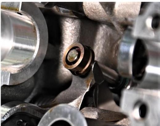
Slide the closing shim up over the half-rings and insure the half-rings remain seated onto the valve stem.
