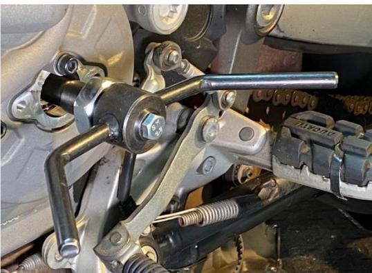
Install engine-turning tool. Remove the cover on the left side of the engine and install the engine-turning tool onto the end of the crankshaft. Note: the tangs on the engine-turning tool fit neatly into indents on the crankshaft. Tighten the bolt to snug and the engine is ready to turn counter clockwise (CCW) into the correct position(s) for valve clearance checking.
