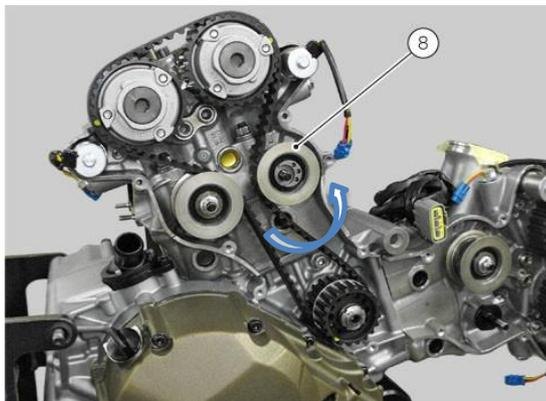
If previously removed, fit the belt tensioner (8), new wave washer, and new Fuji nut. Put slight tension on the belt by rotating the tensioning pulley counter clockwise and gently tighten the Fuji nut. **DO NOT TORQUE** the Fuji nut at this time.
