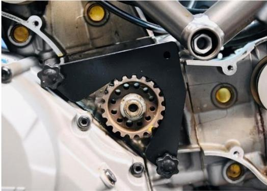
Use the engine turning tool to rotate the crankshaft counter clockwise (by looking at the engine from the left side), to bring the horizontal cylinder piston to the TDC.
