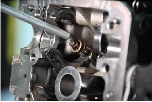
Use the magnet in the kit to remove the half-rings from the valve stem.
