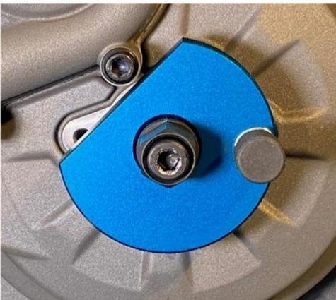
When the timing is correct, remove the engine turning tool from the left hand side of the engine. Install the crankshaft locking tool onto the crankshaft and lock the tool/crankshaft into position.
