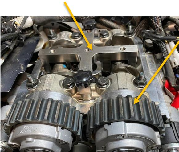
Note: there is spring pressure on the intake cam. Manually rotate the Variator so the flat portion on the camshaft fits neatly into the reaction tool. Use the M6 x 25mm bolts (with plastic knob) to secure the reaction tool to the cylinder head: holding the camshafts in place.
