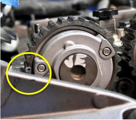
Check the Variator alignment. The marks (dimples) on the Variators will align with the plane of the "head flat surface".
