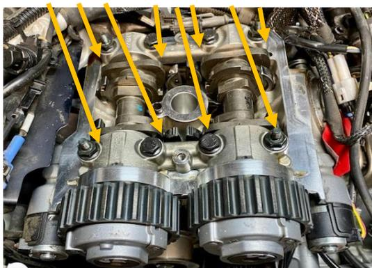
Use gasket sealant on the mating corners where the cam retainers meet the flat surface of the cylinder head for sealing. Torque in two stages to 7ft lbs.
