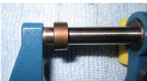
Close the micrometer. Do not over tighten. Press the "zero" button to set the reading to 0.00. Open the micrometer and place the shim on the stationary shaft of the micrometer, with the flat side towards the fixed portion of the micrometer. Measure the opening shim and record the measurement in column [D] of the worksheet. Determine the size of the replacement shim by adding/subtracting column [C] to
