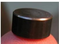
The opening shims are flat on the top and recessed on the bottom so the shim fits securely on top of the valve stem.
