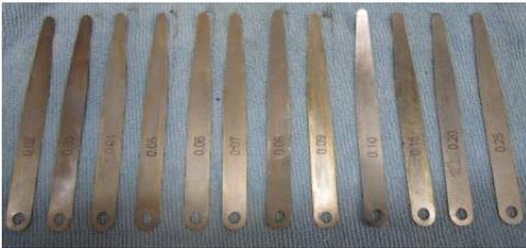
Tip: spread out the feeler gauges in order. This facilitates progressive (larger/smaller) measurement.
