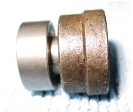
Remember to subtract 10.00 mm from the shim measurement prior to recording the measurement on the worksheet. Record this measurement (minus the 10.00 mm) in column [I] of the worksheet.
