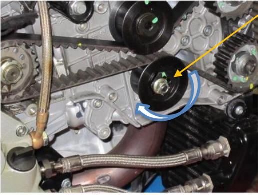
Loosen the tensioning pulley by loosening the Fuji nut and rotating the tensioning pulley clockwise (away from the Variators). Loosen the nut and remove the tensioning pulley from its mounting stud on the cylinder head. Removing the tensioning pulley facilitates belt removal/installation. Label the tensioning pulley (horizontal or vertical).
