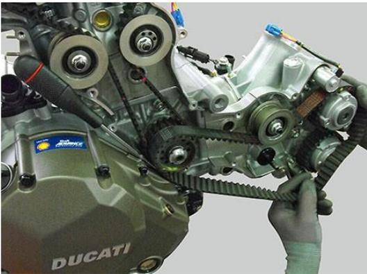
Install the belt for the horizontal cylinder. Place a screwdriver, as shown, to hold the belt in position. If previously removed, fit the belt tensioner, new wave washer and fasten with a new Fuji nut. Do not tighten to torque.
