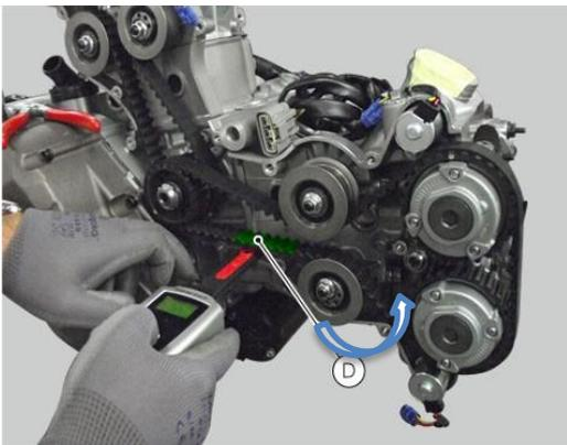
Check the horizontal cylinder belt tension at the indicated point (D). Tension the belt according to the table below.
