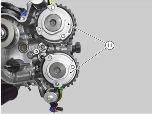
Check the alignment of the Variators (11): the marks (dimples) are aligned with the "head flat surface".
