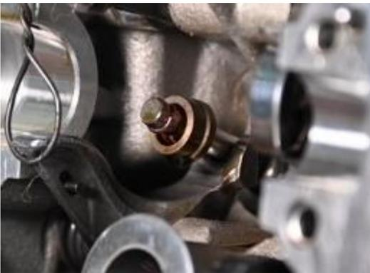
Rotate the half ring to make room for the second half-ring.
