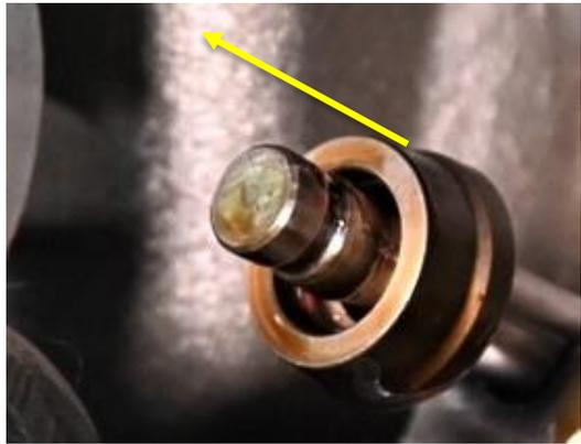
Slide the closing shim up and off the valve stem. Set the half-rings aside making note of their location.
