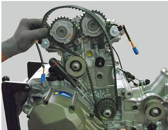
Install the belt on the vertical cylinder: bottom pulley first and work your way up. Use a screwdriver (as shown) to secure it onto the Intermediate Shaft pulley.
