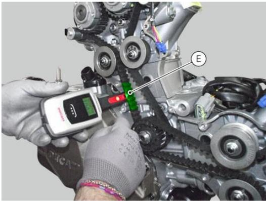
Rotate the crankshaft by 270° counter clockwise to bring the vertical cylinder to TDC.
