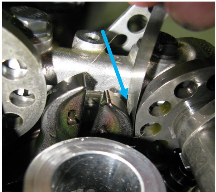
Use the accompanying worksheet (or other preferred method) to record measurements. The worksheet arrangement enables an easy determination about the current valve/shim clearance. It also facilitates determining the new shim size to bring the clearance into specification.
