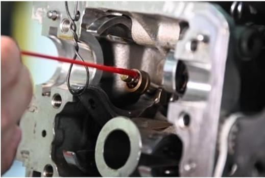
Slide the new shim onto the valve stem.
