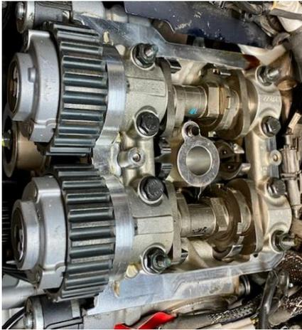
When removing the cam hold-down clamps loosen the inner retaining bolts and then the outer ones. These nuts are ½ the normal height and it is best to use a 6pt socket.
