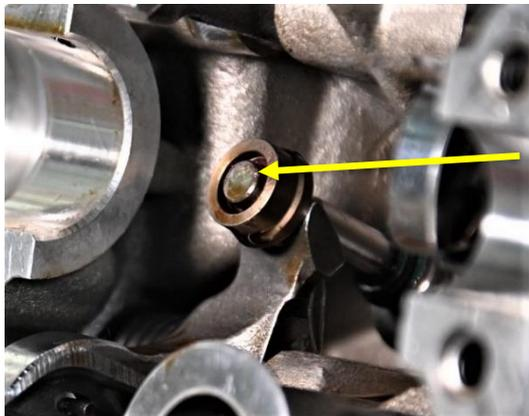
Remove the opening shim by lifting it off of the valve stem.
