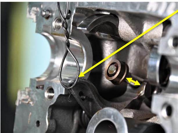
Use safety wire, zip tie, or a screwdriver to lever the closing rocker arm away from the closing shim; relieving pressure on the closing shim. In the photo the closing rocker arm is well away from the closing shim. Remove the opening shim and set it aside.
