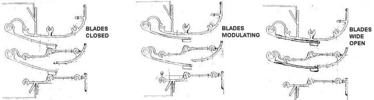
C. Use the information from steps 1 and 2 on the previous page to determine if the damper blades are correct for the conditions.
