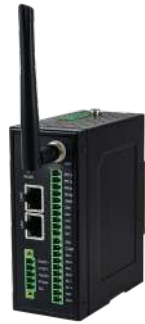
IO5202 with Analog Inputs
