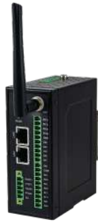
IO5202 with DI0s and Relays
