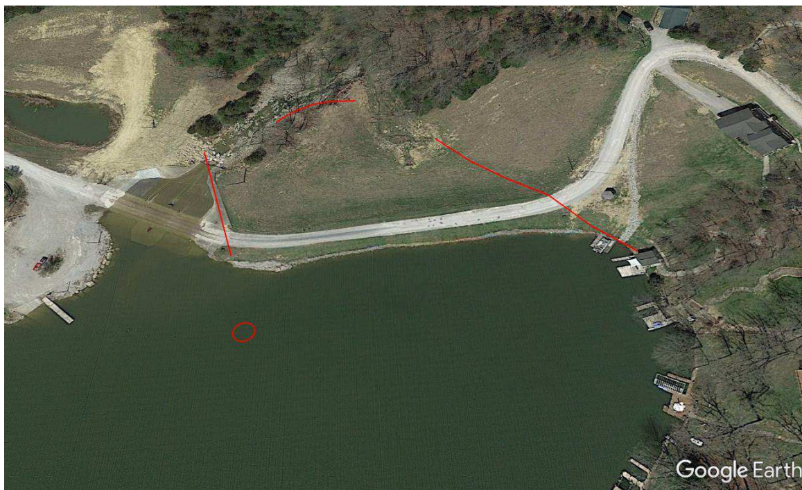
Photo left: The two lines from the lake down the dam are the known leaks. The line along the creek is the exit of a deep leak that we are looking to find the start point.
