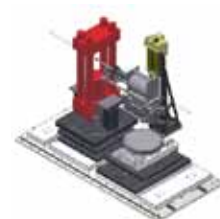
Eleven Axis Custom Design Motion for a Press and a Detector System
