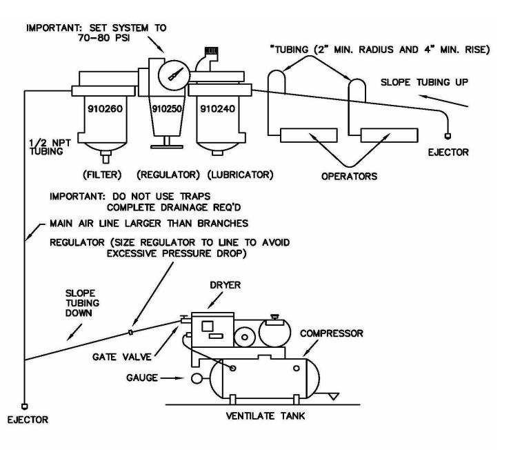
LOCATE IN COOL, CLEAN DRY AREA. DO NOT LOCATE WHERE VENTILATION IS RESTRICTED OR INTAKE WILL HAVE TO BE PIPED TO COOLER, DRYER AREA.
