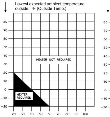
DEGREES FAHRENHEIT Lowest expected ambient temperature at operator power cylinder. (Inside Temp.) FIGURE 1
