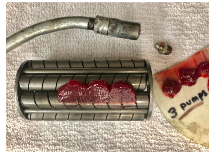
Results from applying grease via the Zerk fitting
