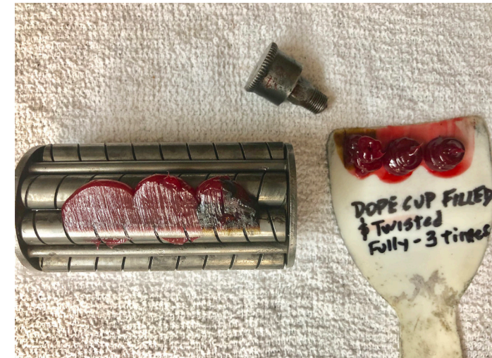
Results from applying grease with the traditional grease cup
