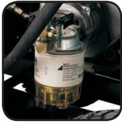
High quality fuel filter/water separator ensures clean fuel supply to the burner
