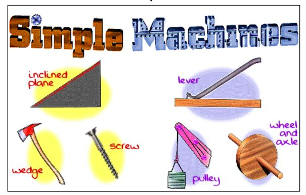
Using these simple machines we apply a: <a href="mailto:small">small</a> force over a large distance to get a:
