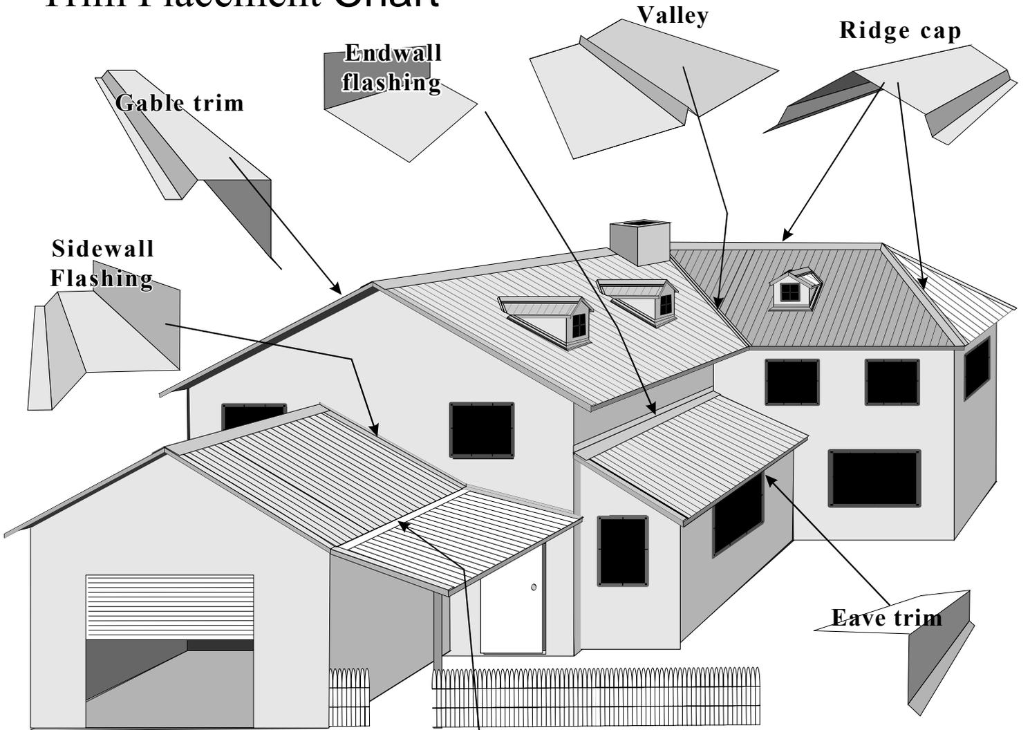
Roofing trims and flashing are named by the location or function of that particular piece on the building.
