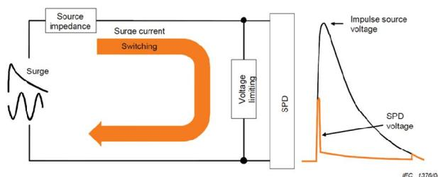
Circuit for voltage-switching devices
