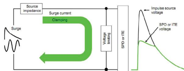
Metal Oxide Varistors (MOV) can withstand high voltages. They have short response time making them suitable for limiting rapidly changing voltages. They can be used in parallel to increase voltage handling capacity. However they have high capacitance. This limits their use in high frequency applications.
