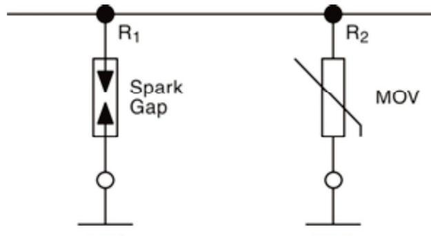
The use of gas discharge tubes in combination with MOVs ( Figure ). This combination of components is associated with lightning test current peak values in the range of 50 kA and voltage protection values of approximately 800 V. Compared to the open-air spark gap, the gas discharge tube is environmentally sealed, has a tightly controlled trigger voltage level, faster response time and a lower discharge surge current rating.
