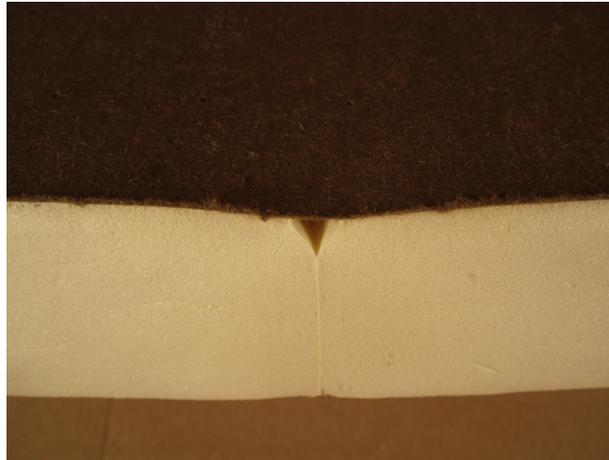
Knit line and V-groove close-up (after conditioning)
