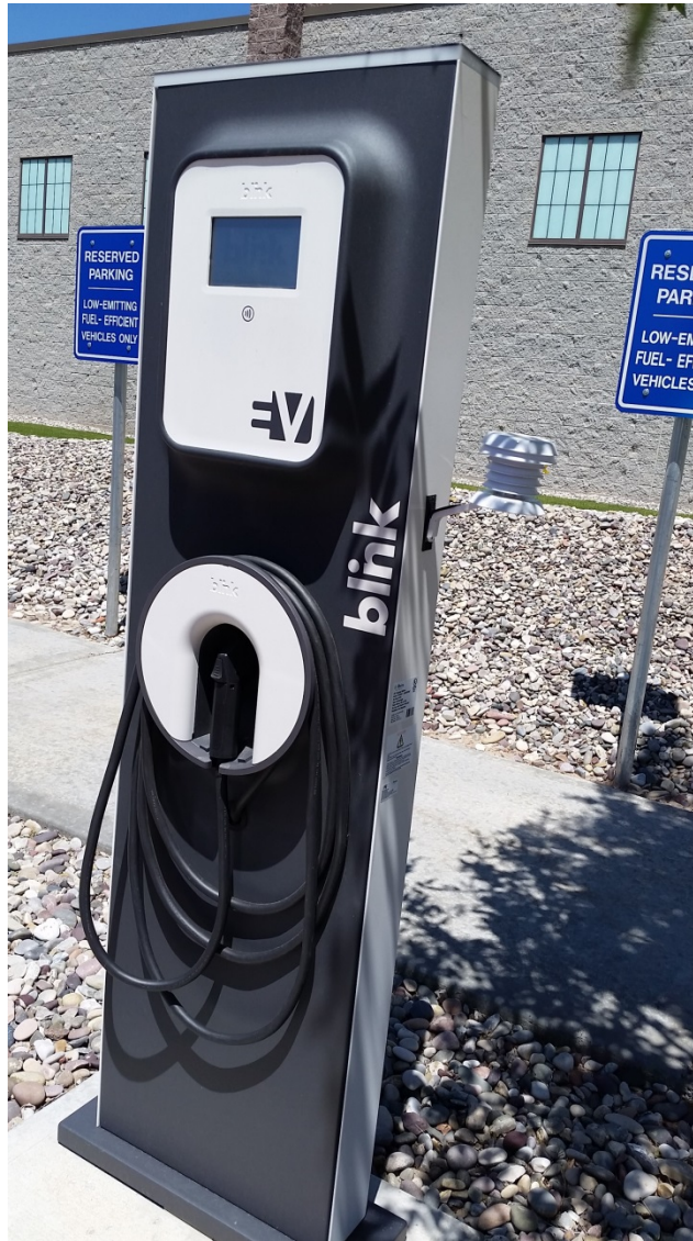
Figure 3. Blink EVSE used during testing, with an attached solar shield for the temperature logger.
