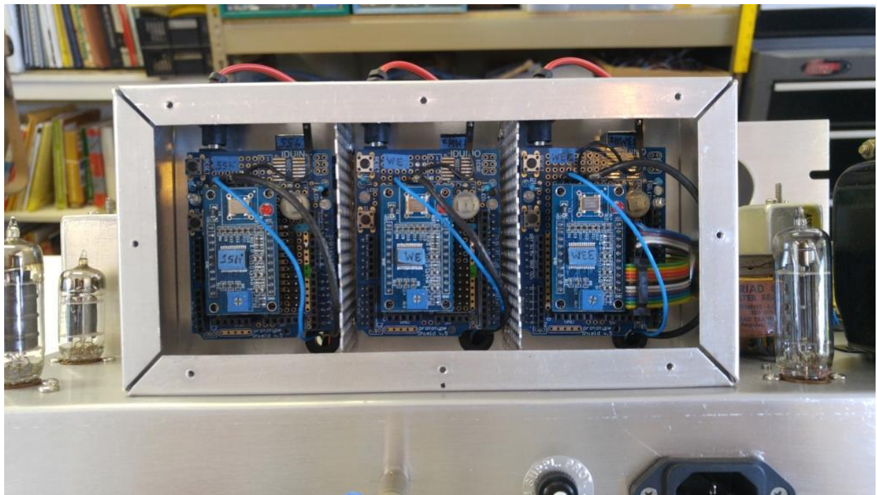
Figure 19: Solid State Chassis in Initial Configuration Three Arduinos and Three AD9850 DDS Modules were Used
