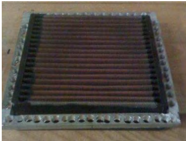
K&N filter with the spacer that Corky used as an attempt to provide more airflow through the air box. Note the filter pleats running left and right (horizontal) in this photo.
