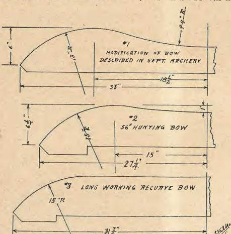
54" long. The eore is composed of one 1/16" lamination of hickory on the back of one of maple 3/32" thick on the face. The backing is 4-ply Glasstox and the facing black Toxhorn. Toxhorn is not recommended for such short bows, but as she draws only 24" it should not be over-stressed. Tufftox would be better, but I had the Toxhorn on hand so used it. The bow came out about 28 lbs. at 24" draw, but by narrowing it down from 1-5/8" to 1-1/2" I arrived at the 24 lbs. she wanted.
