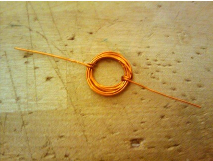
Step2: To keep the coil from unraveling, wrap each end around the coil a few times. The two ends should be on opposite sides of the coil from each other.
