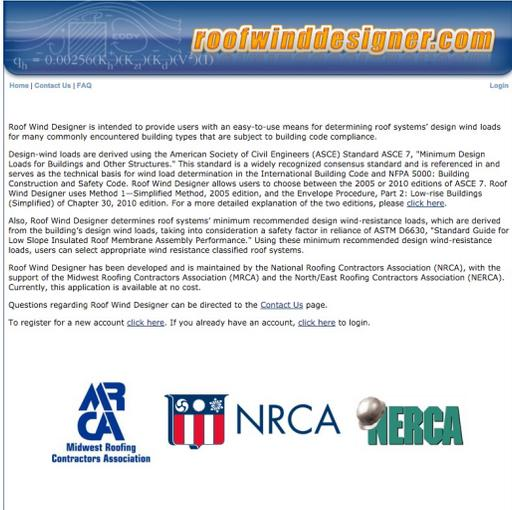
Roof Wind Designer is intended to provide users with an easy-to-use means for determining roof systems' design wind loads for many commonly encountered building types that are subject to building code compliance.
