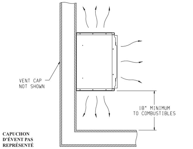
**Figure 1** MINIMUM DE 18" (45.7cm) AUX MATÉRIEAUX COMBUSTIBLES
