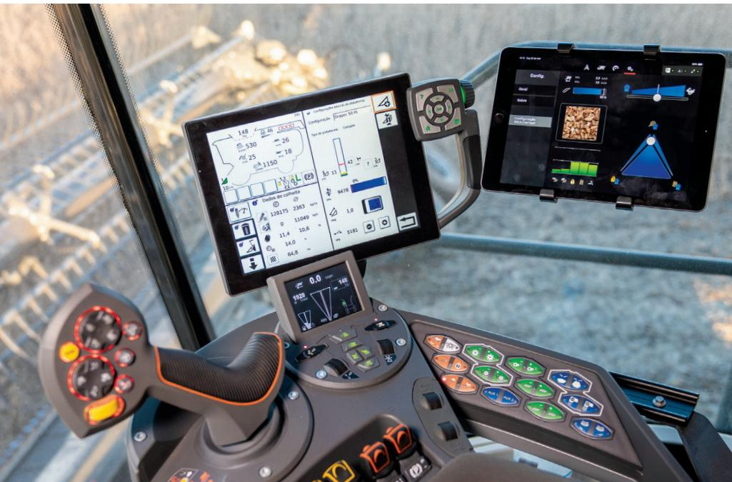
▲ Sensors in AGCO's IDEALTM combine help determine what is grain vs. not, and direct the system to self-adjust on the go.
