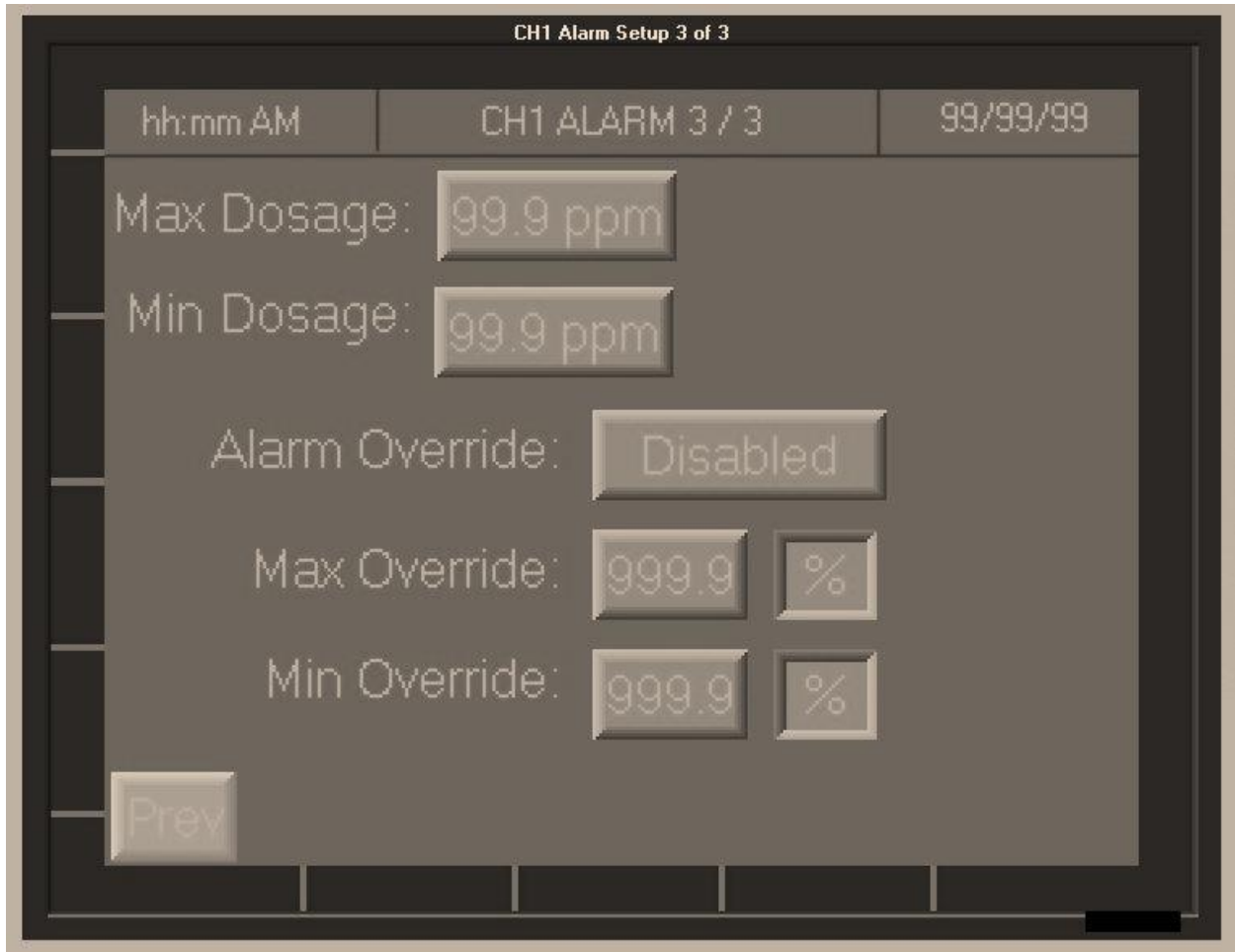
Figure 19: NTL Alarm Setup Screen 3 (of 3) – Dosage Alarm Settings
