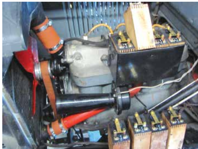
Replacing test coils with previously used coils
