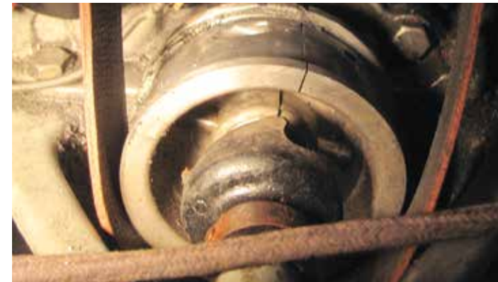
Crank pulley in at 15° past TDC; 3:30-9:30 as hands on clock face
