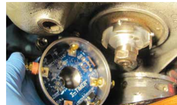
Placing I-Timer case
