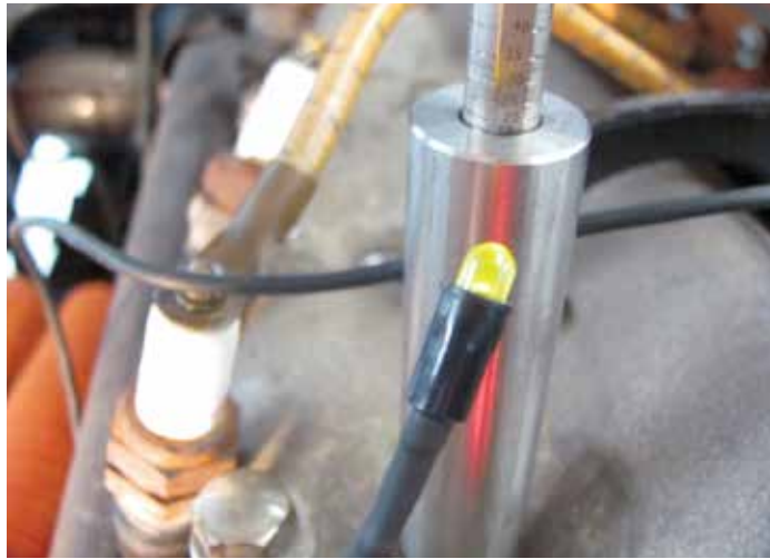
Indicator illuminates at correct timer case setting
