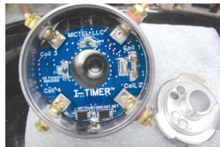
I-Timer case and aluminum rotor
