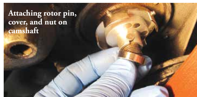
The Accurate Timing Indicator helps to ensure timing is set correctly.
