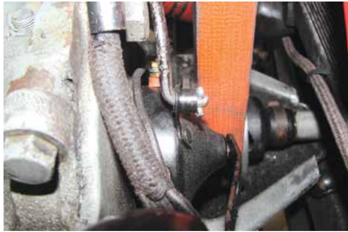
The I-Timer after installation. Looks like a stock timer!
