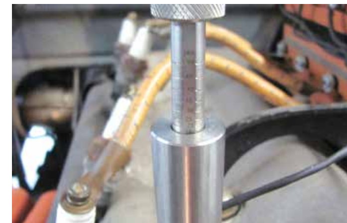
The Accurate Timing Indicator helps to ensure timing is set correctly.
