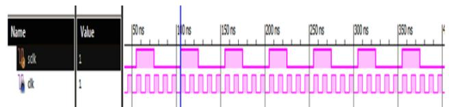
Fig. 6.1: Generation of clock signal of 20 MHz
