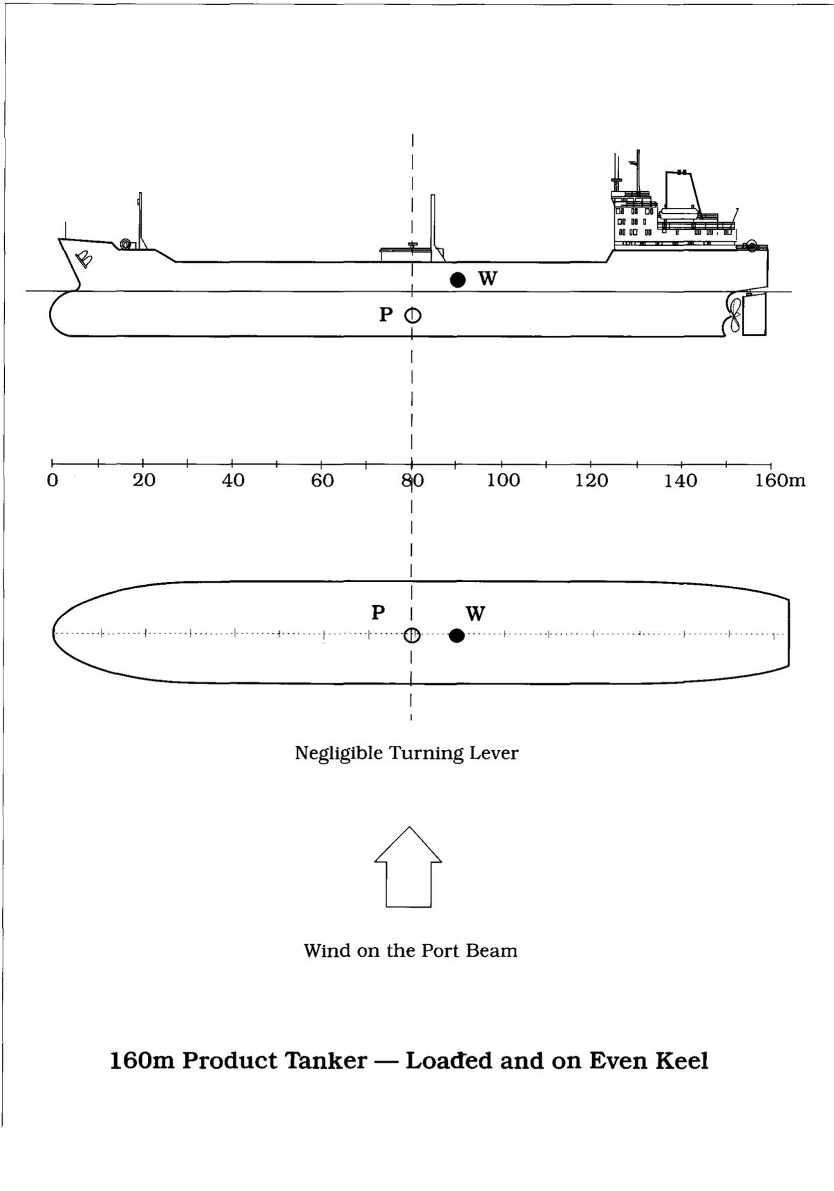
**Fig. 16 Effect of Wind — with Headway**
