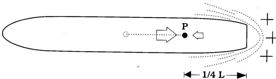
**Fig. 2 Turning Levers and Moments**
