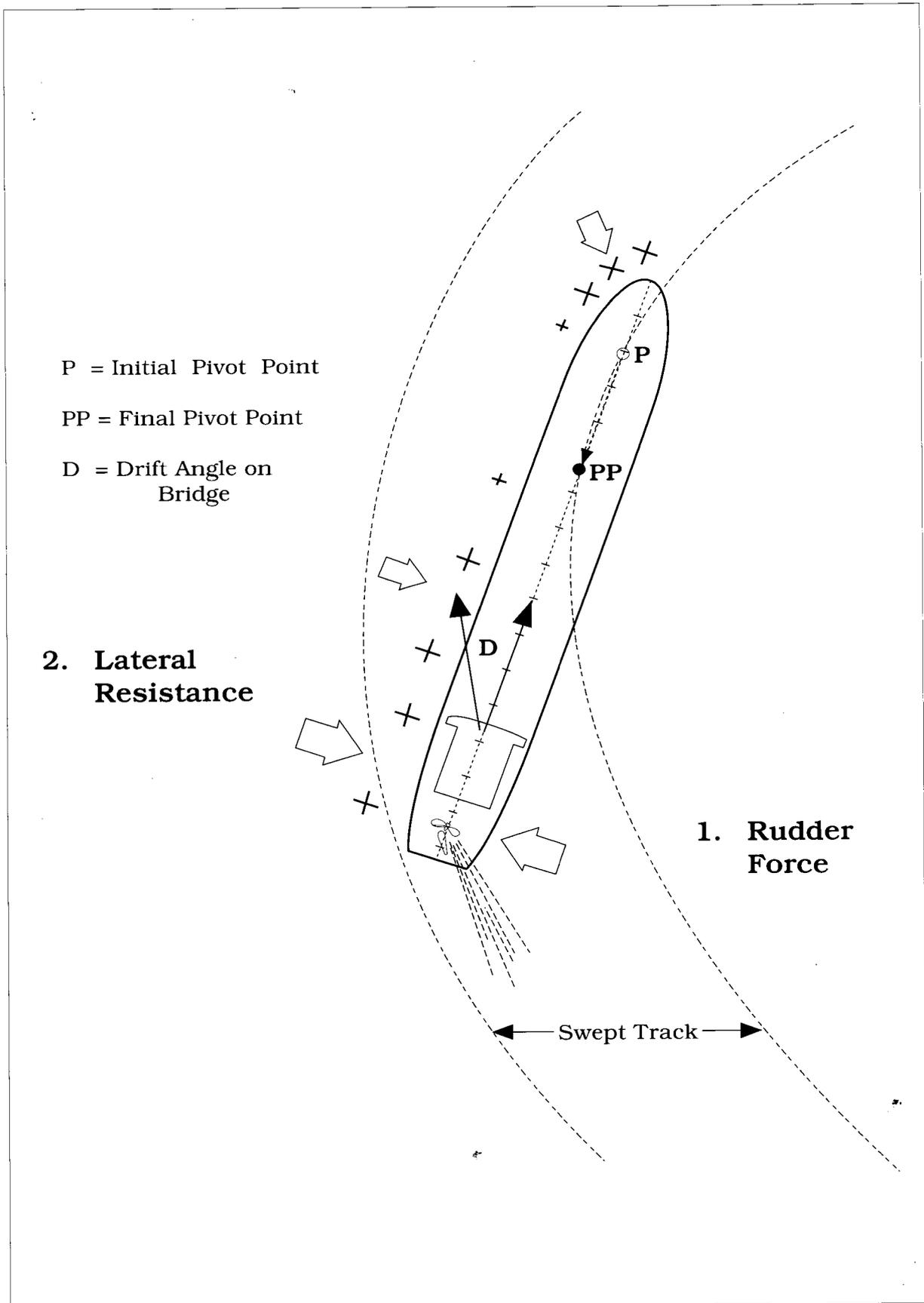
lateral resistance are always achieving the same balance thereby assuring that each turning circle is approximately the same, in terms of advance and transfer. The only thing that is saved by entering a turn at higher speeds is time. It is the 'rate of turn' which varies. Whilst this can be critical in cases when time is of paramount importance, such as conducting a large turn across a strong tide or taking the ship through a 'Williamson Turn', it does not improve turning ability.
