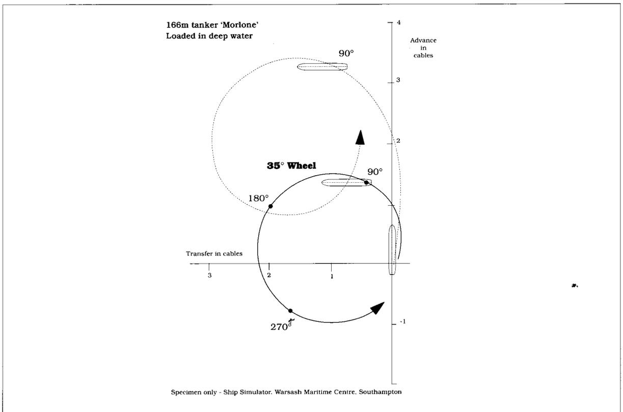
handling characteristics and in particular its turning ability. **As a rough guide it can be assumed that a ship may experience shallow water effect when the depth of water is less than twice the draft**, i.e. the under keel clearance is less than the draft itself. Serious cases of shallow water problems have however, been experienced with larger under water clearances, especially at high speeds, sometimes with dire consequences!
