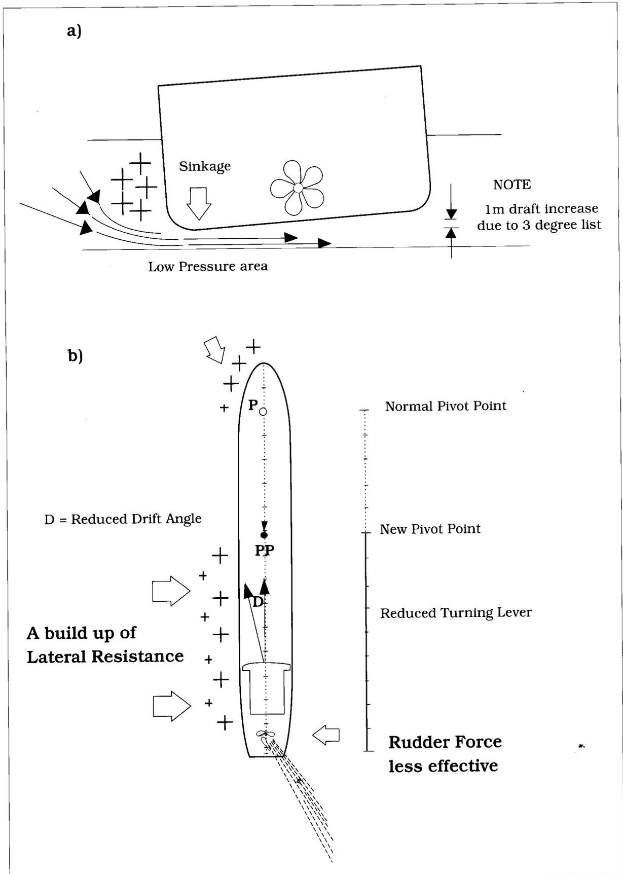
**Fig. 13 Turning in Shallow Water**
