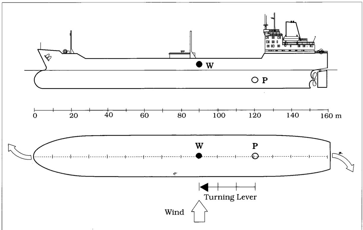
When, however, approaching a berth or a buoy with the wind dead ahead with the ship on an even keel, the approach should be much easier to control. Even at very low speeds the ship is stable and will naturally wish to stay with the wind ahead until stopped.
