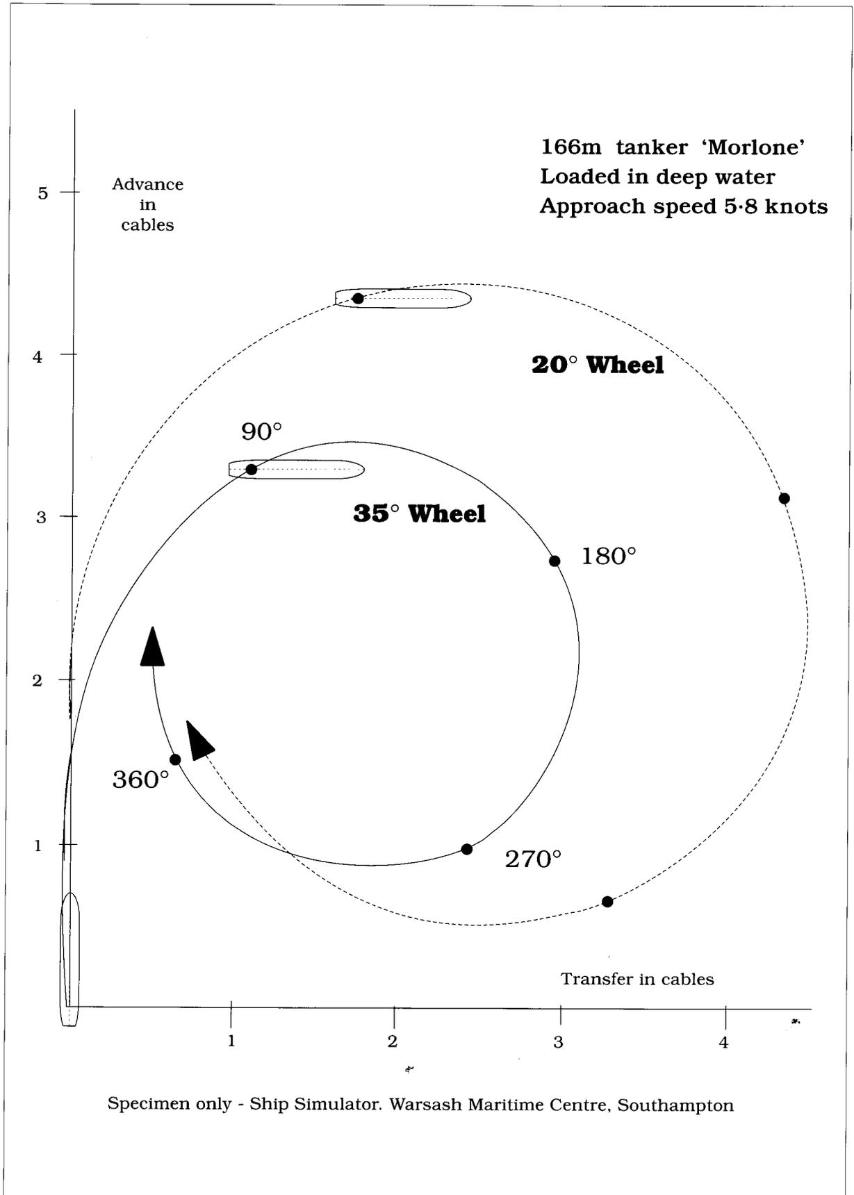
**Fig. 9 Full Ahead Turns to Starboard**
