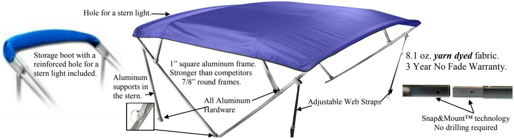
8' x 8', 4 Bow Economy Pontoon Top fits boats with 8' wide decks. 1" Snap&Mount™ square frame with mounting hardware included. Top installs with four zippers. Stern Supports and Storage Boot are Standard. Front secured with straps. The pontoon top fabric mounts with zippers, less hassle with assembly, and zips off for winter storage. The frame snaps together in minutes.
