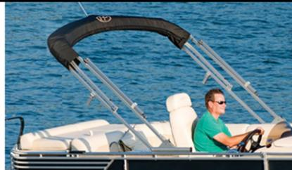
Folds into the storage position or flat. 1 1/4" satin finish anodized frame.
