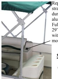
Replace front web straps with the durability of aluminum strut bars. Fully adjustable from 29" to 34" in length / with aluminum mounting hardware.
