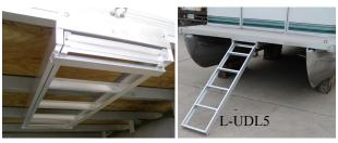
Five step extends 59" below the deck. Rated up to 300 lbs. Stows under the pontoon deck when not in use.
