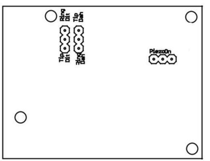
the header, long pin into a breadboard, then place the PCB over the short pins and solder in place. This ensures the header is mounted square and makes for a neat result. Once the header blocks are in place and you are happy with the alignment. Find the 2 diodes (1N4148) and insert in the board. Make sure that the black band of the diode body matches the line printed on the PCB. Both diodes face or point the same way. Solder in place, see the diagram below:
