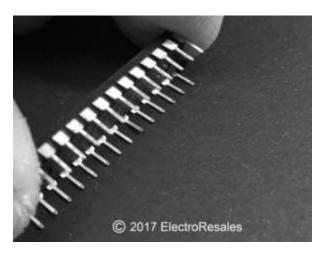
Then, applying an equal amount of force to the pins, bend them in slightly. This process does not need a lot of pressure. Once the pins are properly in line, line the IC up with the socket and insert, make sure to have the notch on the IC line up with the notch on the IC holder. Check that all pins are in the socket and none are bent under.
