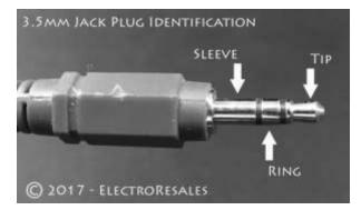
The Dit paddle can be wired to either the Tip or Ring and the common to the Sleeve, likewise the Dah paddle can be wired to either the Tip or Ring. Whichever way you choose, set the jumpers to reflect your choice by using the shorting links to short the middle pin and the respective outer pin for Tip or Ring per the legend on the PCB on each header. For example if the Dit paddle is wired to the Tip, then the Dah paddle is wired to the Ring. Set
