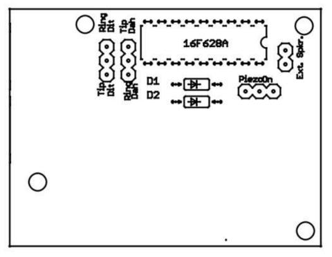
This diagram shows the IC holder in place and the direction of the notch, arrowed;
