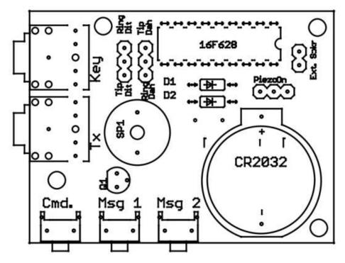
After checking the parts take a look at this diagram to get an idea of the parts placement/positions before soldering any parts. It shows clearly the major components.
