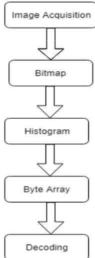
Fig 3: Detecting 2D barcodes
