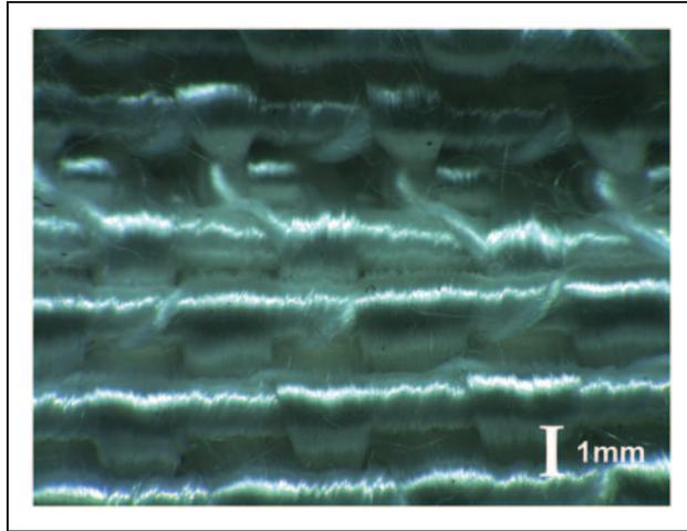
**Figure 3.** Fabric B comprising helical auxetic yarn B as warp fibres (horizontal).
