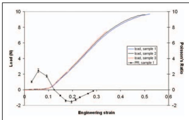
**Figure 12.** Variation of tensile load with strain for three samples of yarn C, overlaid with Poisson's ratio of one sample.
