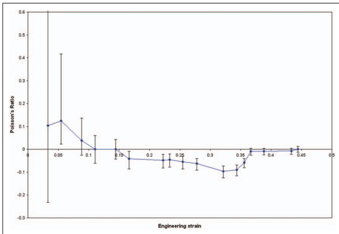
**Figure 18.** Variation of Poisson's ratio with longitudinal strain for fabric B.
