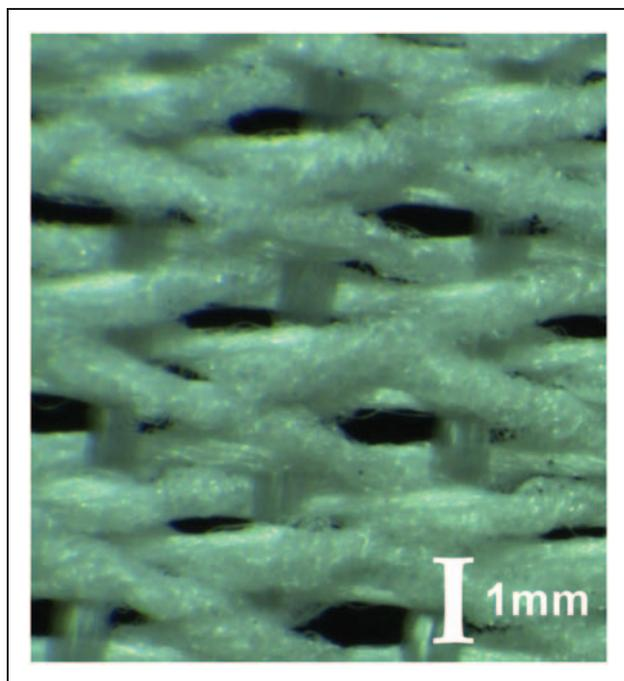
**Figure 15.** Fibres overlap, giving rise to negative Poisson's ratio out-of-plane and a consequent reduction in in-plane negative Poisson's ratio.
