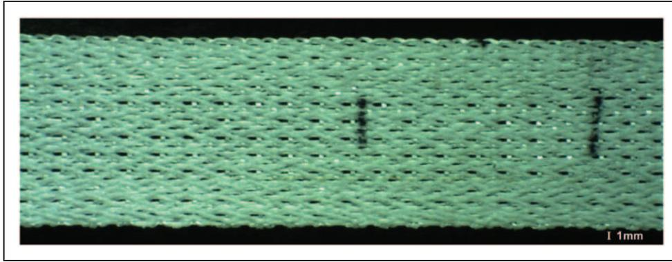
**Figure 13.** Fabric C at approximately 30% strain, showing open pores and gauge markers.
