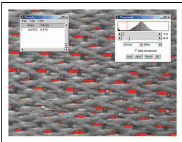
Figure 8. Measuring the proportion of open area of fabric at a given strain. The *Threshold* slider is adjusted until the open area is judged to be precisely represented by the red mask. Then the area is measured (indicated in the *Results* window).
