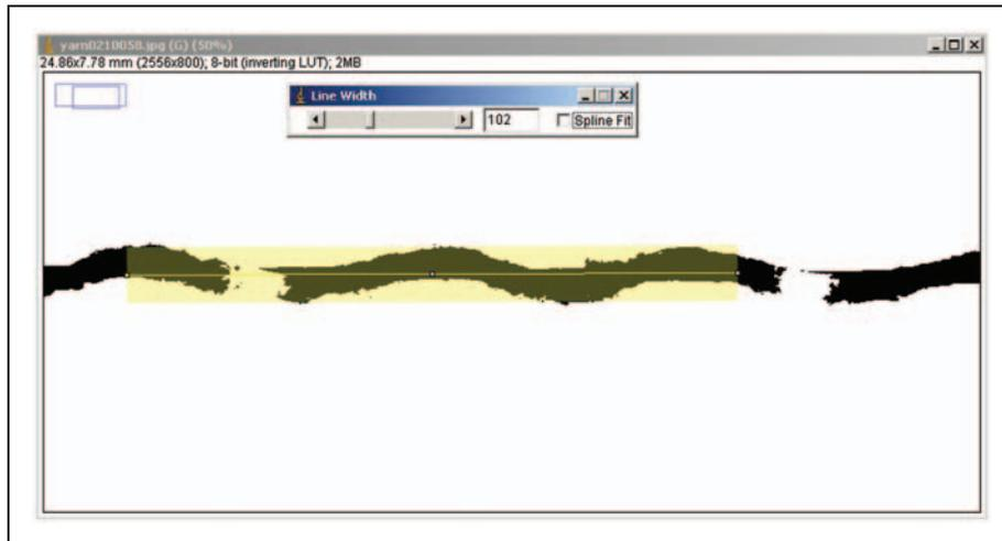
Figure 7. Measuring effective diameter of a helical auxetic yarn.
