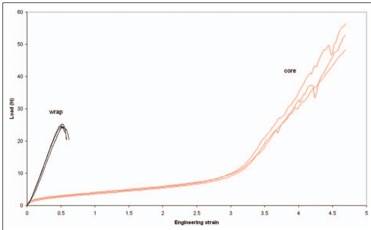
Figure 9. Load-strain data for three samples each of yarn A core and wrap components.
