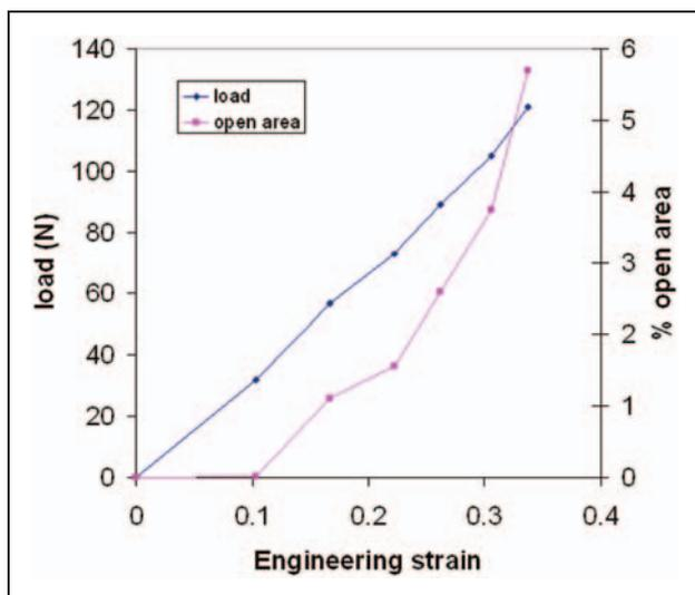
**Figure 16.** Variation of fabric percentage open area and load with strain for fabric C.
