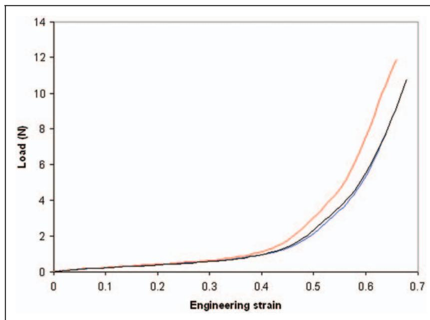
**Figure 11.** Variation of tensile load with strain for three samples of yarn B.
