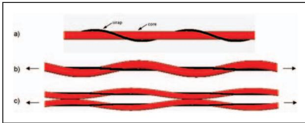
**Figure 1.** a) Components of the helical auxetic yarn (HAY); b) auxetic behaviour under tension; c) fabric application – pores open under tension in a complementary pair of HAYs.
