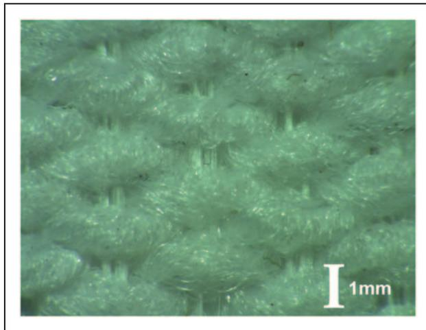
**Figure 4.** Fabric C comprising helical auxetic yarn C as warp fibres (horizontal). (The fibrous nature of the textured nylon wrap obscures the HAY structure.)
