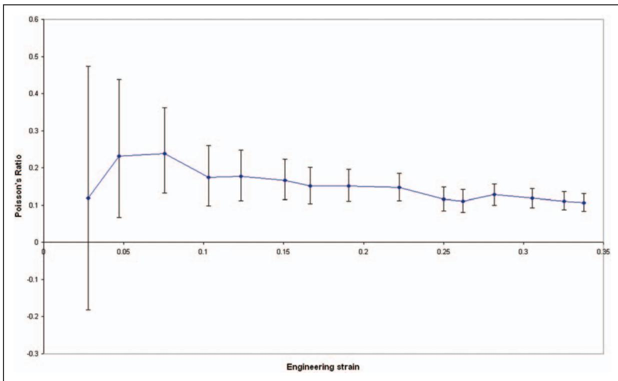
**Figure 14.** Variation of Poisson's ratio with longitudinal strain for fabric C.
