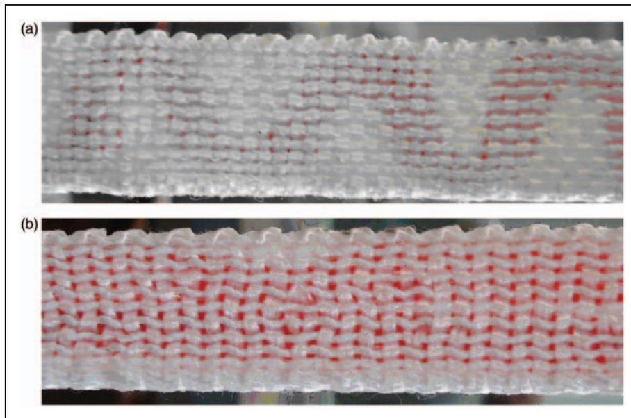
**Figure 17.** Prototype colour-change fabric B; a) 0 N tension, b) 80 N.
