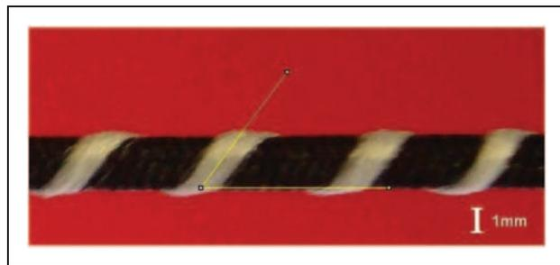
**Figure 5.** High-resolution image of helical auxetic yarn A during tensile test and subsequent measurement of wrap angle.
