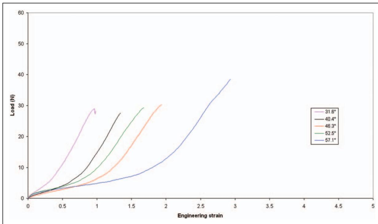
Figure 10. Measurements of the effect of initial wrap angle on strain-dependent behaviour of yarn A.
