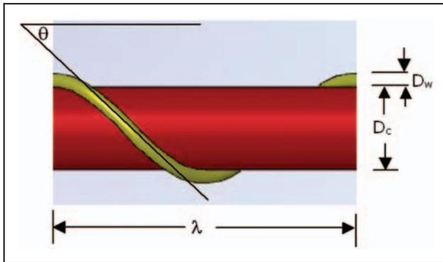
**Figure 2.** Geometry of the helical auxetic yarn.
