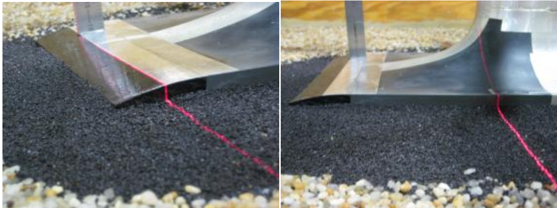
55 56 Figure 7. Gravel level after flume test for 12.7mm high 57 elevation with a 12.7mm high straight-sided curved leading edge 58 ramp. No scour is observed (7).
