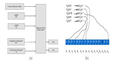
Fig.6.2: Basic bloom filter functionality
