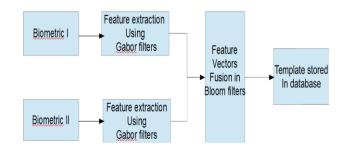
Fig.7.1: Gabor filter based multi biometric template protection
