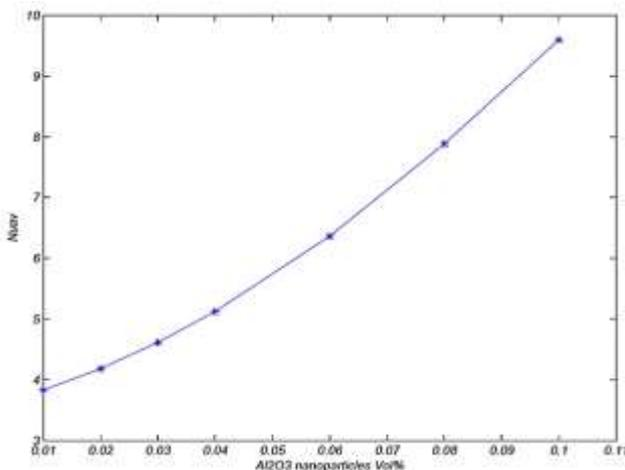
Figure 3. The effect of Al<sub>2</sub>O<sub>3</sub> nanoparticle concentration on the convention heat transfer coefficient of nanofluid
