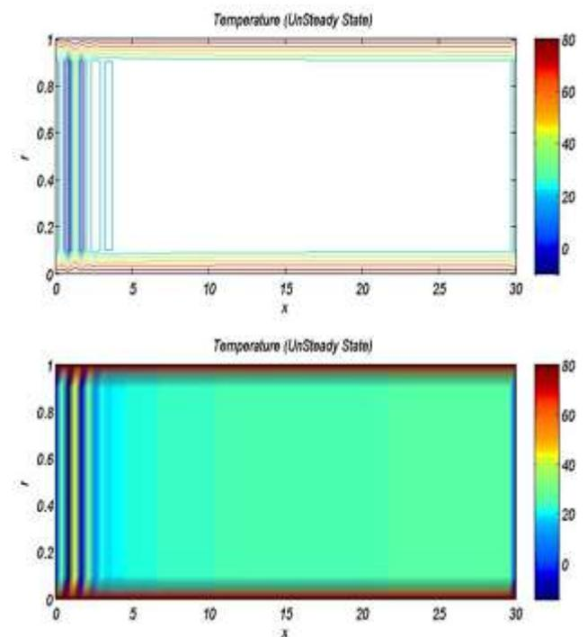
Figure 2. The nanofluid temperature field containing 5 % (v/v) of Al<sub>2</sub>O<sub>3</sub> at Re =885 and the surface temperature of 80°C
