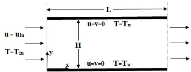
Figure 1. Flow in a cylindrical Duct with a length/diameter ratio of 30.
