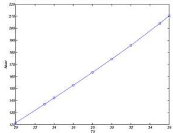
Figure 5. The effect of the fluid inlet temperature on the convection heat transfer coefficient in Re = 450, 4% vol of Al<sub>2</sub>O<sub>3</sub> and the constant surface temperature of 80 ° C in cylinder
