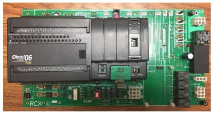
RCX is a drop-in controller upgrade kit for Remstar vertical carousels. The kit includes a PLC and adapter board with pin-compatible interface connections to the existing Remstar control panel cables and components.
