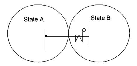
Case-2: Interconnecting line owned by State-B Metering point: Substation of State-A
