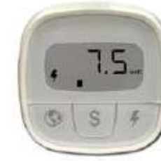
EC Motor @ Low Speed Watt Usage
