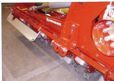
3 point linkage cat. 3 with floating lower links.
