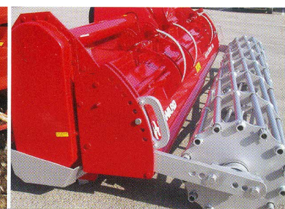
Compact depth control system for rear wheels and rollers.
