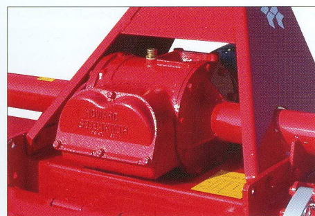
R600B-S The selectatilh gearbox is very reliable and suitable for tractors up to 140 HP.
