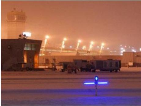
Luminaerospace, LLC demonstrated this new lighting fixture at Ohio's Cleveland Hopkins Airport (CLE) for over a year, through all weather conditions. The system allows Pilots to intuitively recognize the actual pavement edges at night and/or in inclement weather. Additional enhancements have been made that allow advanced cockpit displays to detect infrared light for heads up displays and night vision goggles. The new lights improve pilot situational awareness even in good weather.
