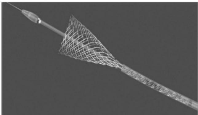
**Figure 1.** The Carotid Wallstent is a self-expanding stainless steel stent with a monorail delivery catheter system that contains a 5.0F to 5.9F shaft. The stent is available in diameters of 6, 8, and 10 mm and lengths of 20, 30, and 40 mm.
