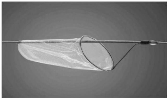
**Figure 2.** FilterWire EX/EZ emboli protection device with a suspended radiopaque nitinol loop, filter pore size 110  $\mu\text{m}$ , sized for 3.5 to 5.5 mm–diameter vessels. The device is compatible with 0.014-inch guidewire.
