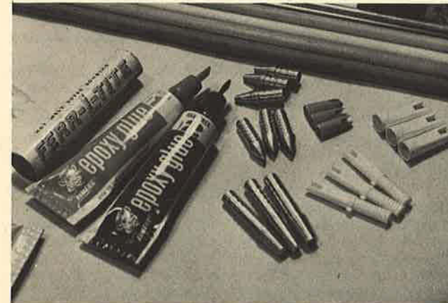
Above: The inserts used in fiberglass and aluminum shafts are held with a solution of epoxy or the Ferr-L-Tite hot melt stick may be used in completing the set of arrows.
