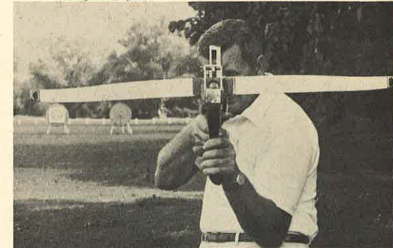
BELOW: Gurik demonstrates the novel submachine gun grip, which he designed to give him a steadier hold on target.
