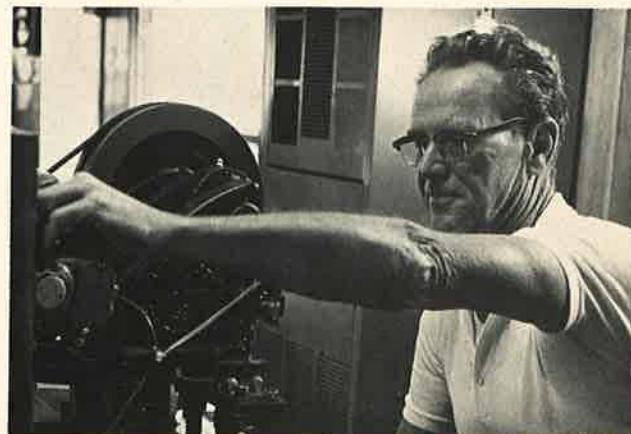
After the counter is reset on the machine, the plastic is lined up, a switch is thrown and the cuts are made.
