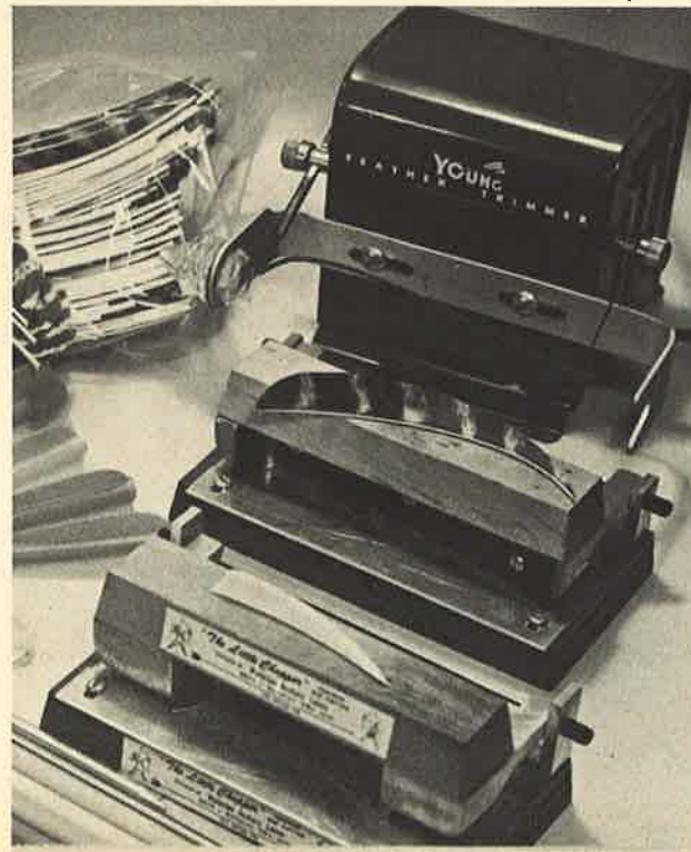
Below: The unit in foreground is the Little Chopper for shaping the fletch. In rear is the Young Feather Trimmer, which uses a heated wire to burn the feathers to shape.
