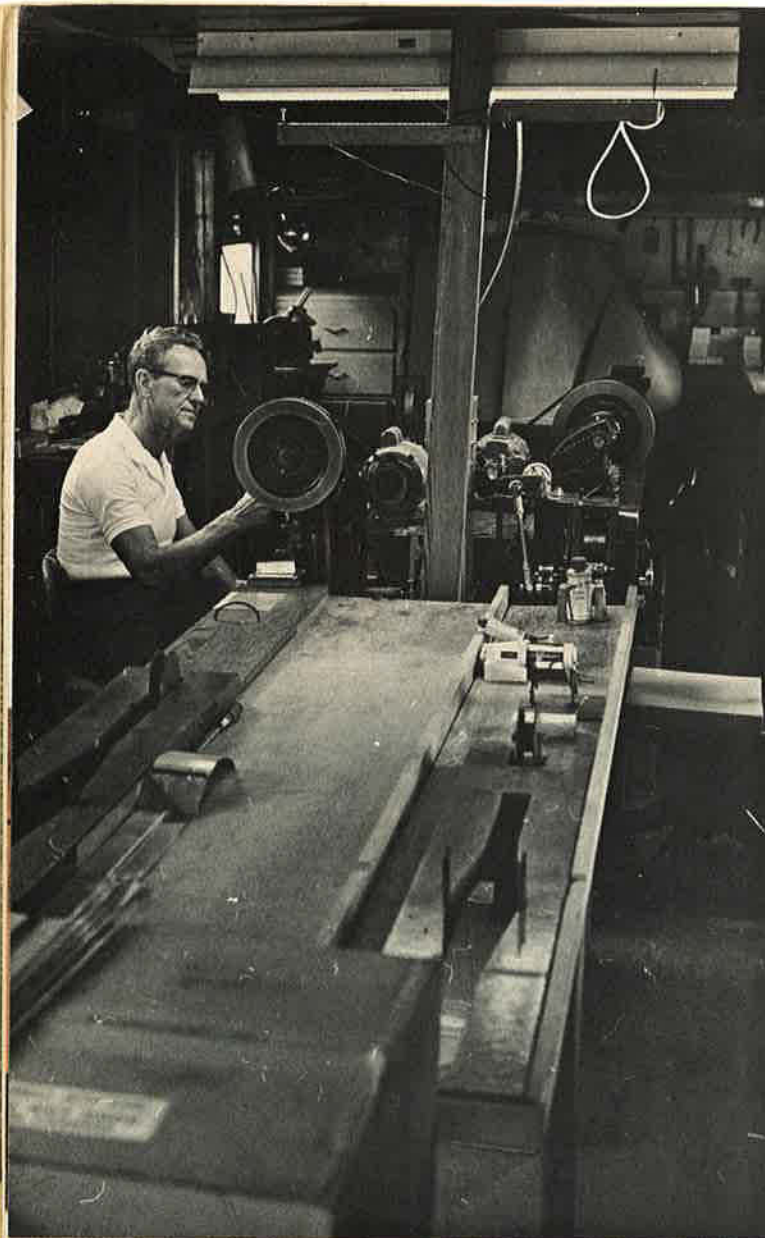
Hamilton gave up the spotlight of the bandstand for the work light over his bench, where he runs a new batch of Plastifletch. (Below) The machine is reset for another run. It takes 21 seconds to cut a hundred of the vanes.
